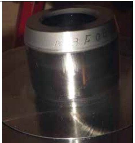
No cavitations found directly on damper
