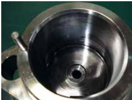
Fig. 50: Fuel valve with guide rings. Inspection after 2,000 hours in service on an S90ME-C9.2
