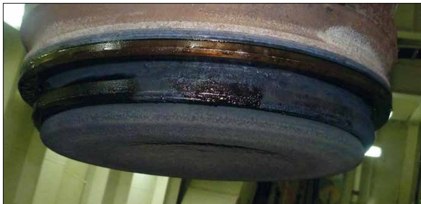
S60MC-C8: Running hour 26,000 Burn away: >11 mm (max. 9 mm)
