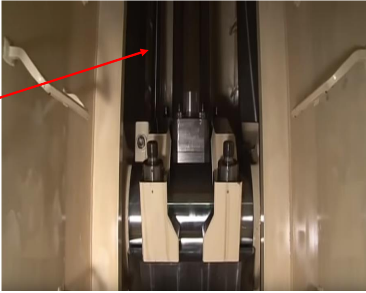
TELESCOPIC LUB. OIL PIPE CONNECTED TO THE CROSSHEAD SLID SHOE
