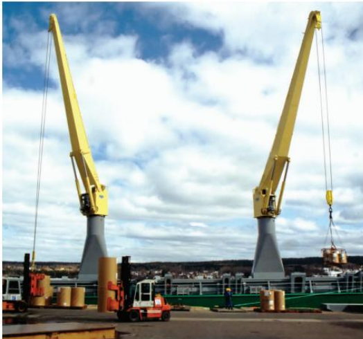
Applications: Cargo handling on container ships, reefers and general cargo ships. Low built.
