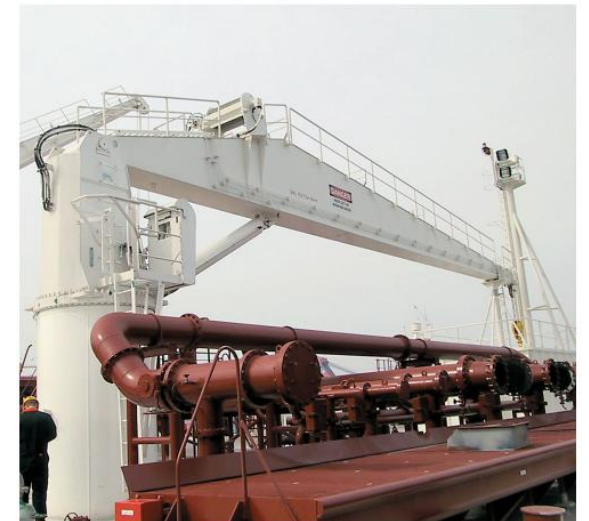
Applications: Handling heavy and multi-purpose cargoes on general cargo ships. Variable frequency drive (VFD) or electro-hydraulic drive.
