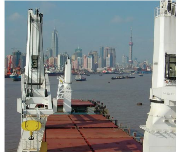
Applications: Handling heavy and multi-purpose cargoes on general cargo ships. Variable frequency drive (VFD) or electro-hydraulic drive.
