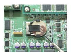
6) Insert the flat tip **nonconductive** screwdriver for adjustment or some stick to the location shown in the figure below and slide the battery sideways to remove the battery.
